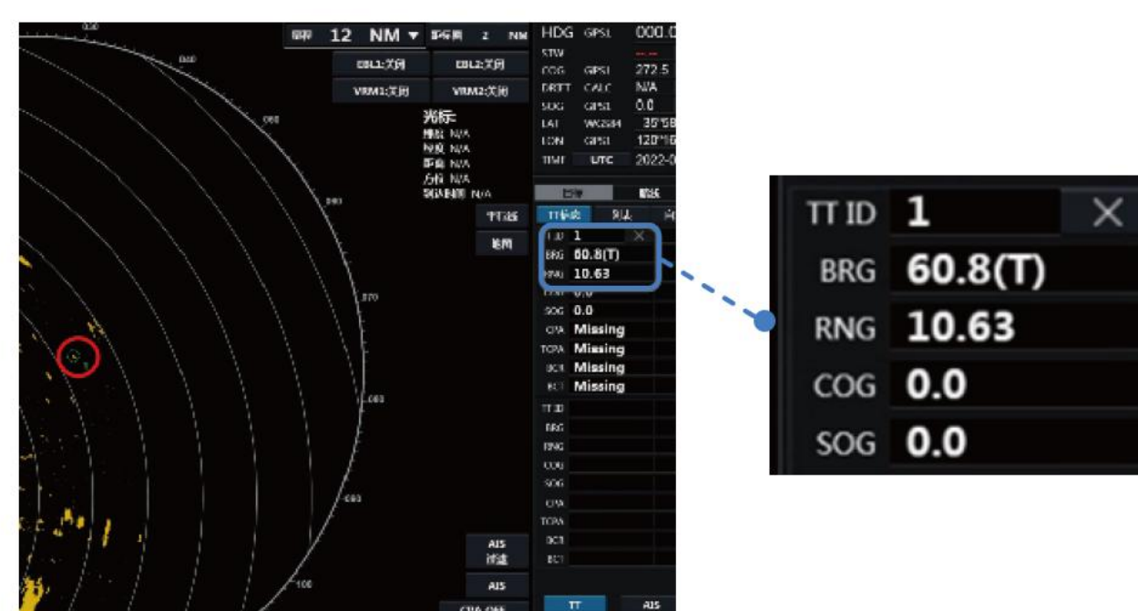
Detection range of a standard 10m 2 sphere at X-band (IMO standard 4.9NM)
